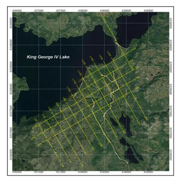
Figure 9.7 An orthophoto of the King George IV Lake area overlain with TRU's 2021 Induced Polarization survey grid. Source: TRU Precious Metals Corp. (2023).
